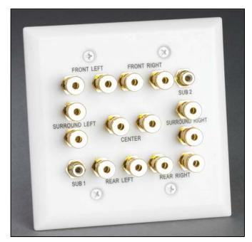
It is important to leave enough excess wiring in the wall to help reduce the amount of tension to each termination. Keep speaker wires and RCA cables away from AC wiring. If these wires must occupy the same area, keep them as far apart as possible and have them cross at a right angle when crossing is necessary.
